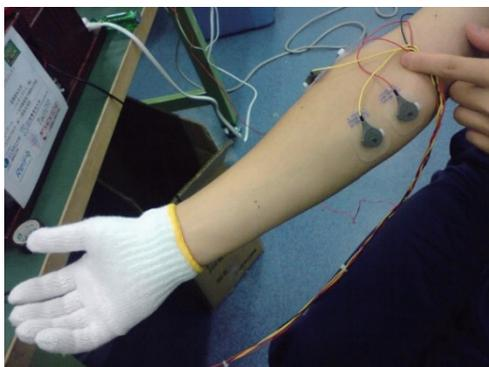
Fig. 3. (Color online) Positioning of myoelectric sensors.
